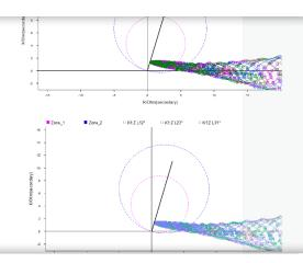
Conducted lab testing to evaluate the actual performance of transmission protective relays under stable and unstable power swings.
