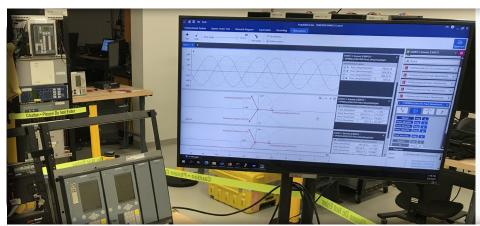
Developed testbed systems and conducted independent technology assessment of process bus technologies and solutions
