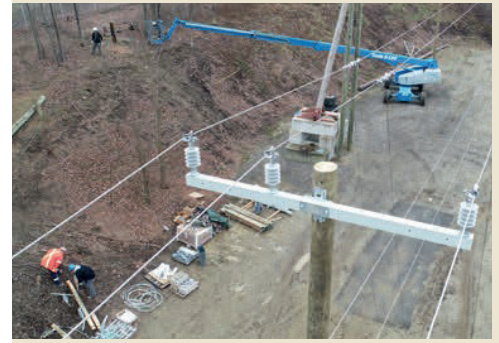
The full-scale overhead structure test facility exposes lines to midspan tree strikes to investigate structural failure modes and identify opportunities to improve structure resiliency.
